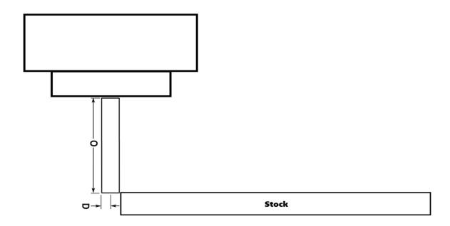
Step 2: Jog pin/finder to touch X and Y axis off part. Use the directional buttons on the controller and once you get close to the stock you will select the:
