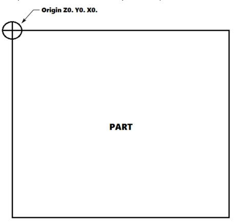
Next place your tool (endmill ect.) in collet and touch off in the Z axis and zero Z axis with the same features.
